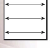
With your steel tape, measure from the inside opening from the left side to the obstacle that projects furthest from the right side of the window. Take this measurement at the bottom, middle and top of the window opening. Select the narrowest of measurements as the correct measurement. This will give you the measurement which will determine the width of
